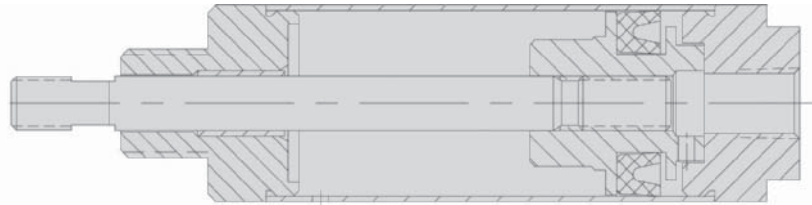
SINGLE-ACTING AIR CYLINDER.
