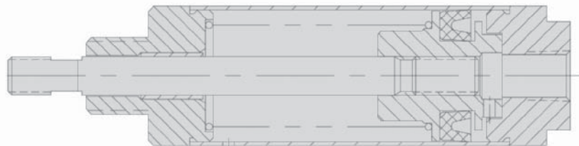
SPRING RETURN SINGLE-ACTING AIR CYLINDER.
