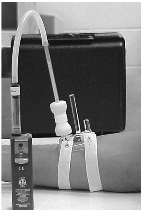
Figure 10.4 Apparatus for trapping volatiles from a human forearm in vivo (Saiyasombati and Kasting, 2004a).
