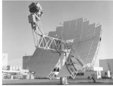
Fig. 1 Faceted parabolic mirror system developed by SES and the US Department of Energy [7].
