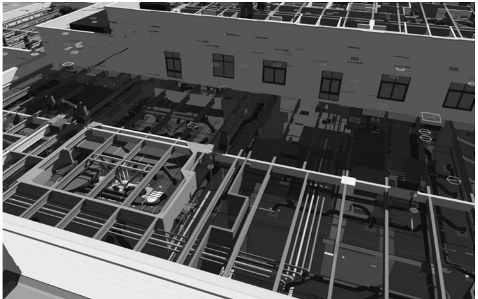
Figure 2.25 Construction model of Sutter Surgical Hospital North Valley. Overall coordinated systems. (Image courtesy of RQ Construction.)
