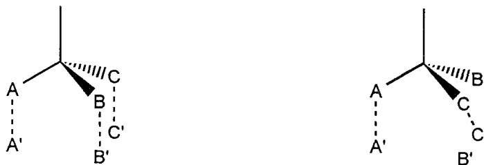
FIGURE 7.2 The three-point theory to explain stereoselective selection in chromatography. One isomer can interact closely with all three binding centers: the second isomer can only interact closely with two binding centers at any one time.
