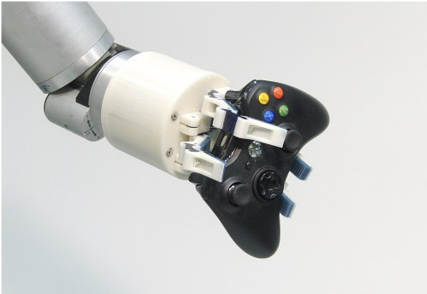
Figure 10: The SDM Hand (source, Dollar and Howe 2010).
