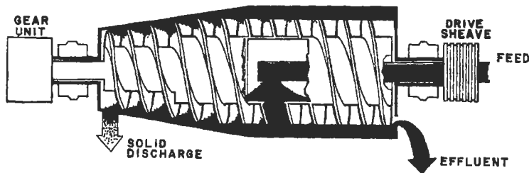
Figure 11. Continuous solid-bowl centrifuge.
