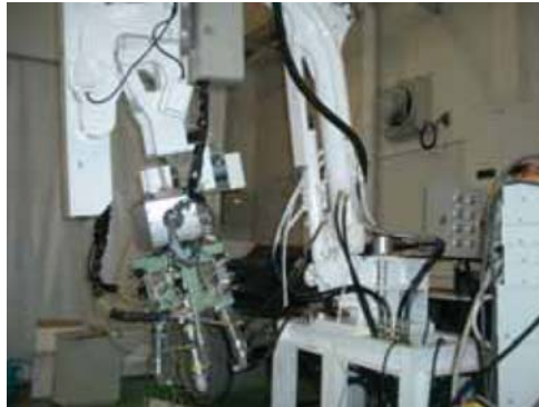
Figure 20. Overview of slave hand system for master-slave bilateral hand system for mine clearance.
