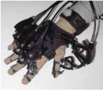
Figure 21. Master hand as human hand with a data-glove and with an exoskeleton.
