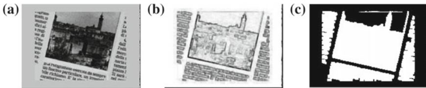
Fig. 9.3 a Original document image. b Image resulting from the inversion of the fuzzy gradient image. c Extracted connected components
