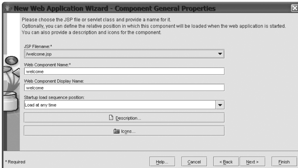
Figure 3-6. The Component General Properties dialog box allows you to select which JSP is being configured. If your application has multiple JSPs, you can rerun the wizard multiple times and select a different JSP each time.
