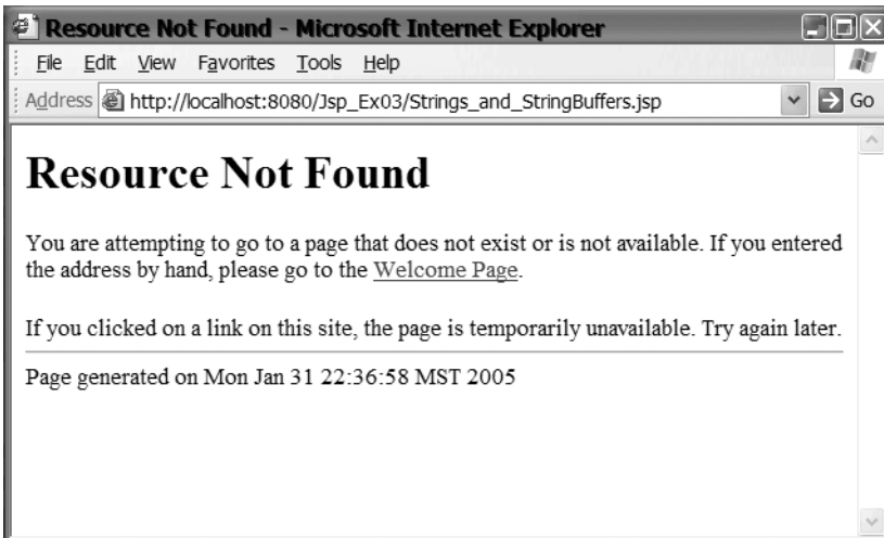
Figure 3-22. When the String and StringBuffers page cannot be found, NoSuchPage.jsp is called.
