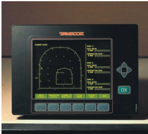
FIGURE 6.2.-25. Hole position and drill angle instrument user interface (TCAD).
