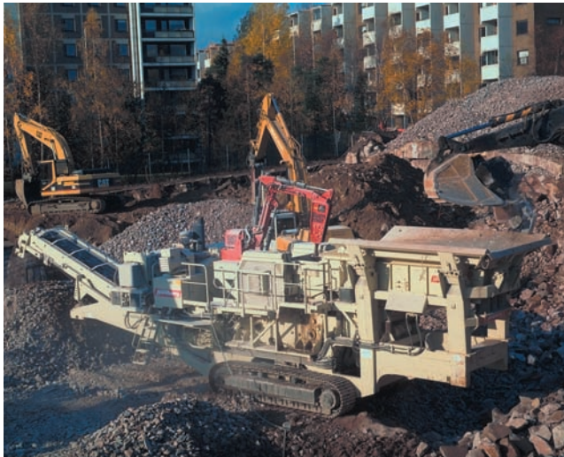
FIGURE 3.9.-10. Nordberg LT110 track-mounted primary crushing unit can be easily moved around a building site as excavation work progresses.
