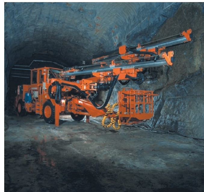
FIGURE 6.2.-22. Wheel-mounted drilling rig.
