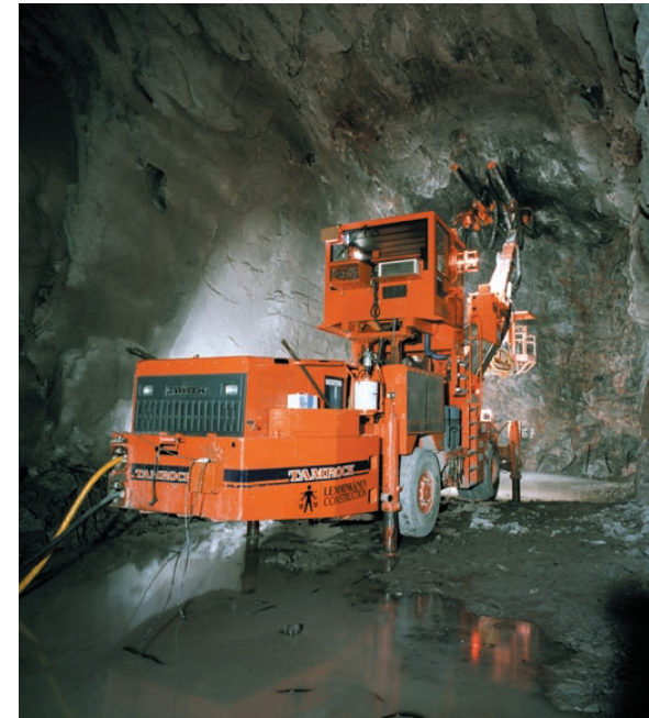
FIGURE 6.2.-26. A fully computerized drilling jumbo.
