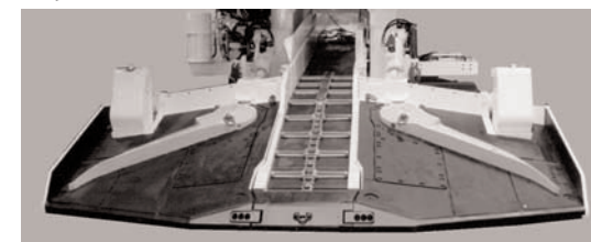
3 Two lateral loading beams
