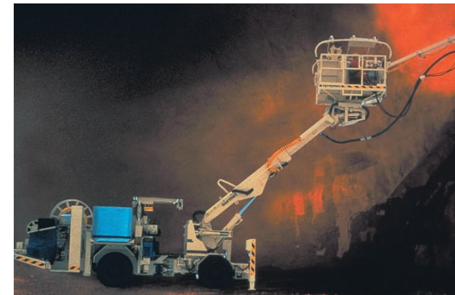
FIGURE 6.2.-73. Mechanized shotcreting unit.
