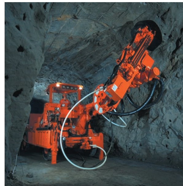
FIGURE 6.2.-71. Tamrock Cabolt. A fully mechanized cable bolting unit.
