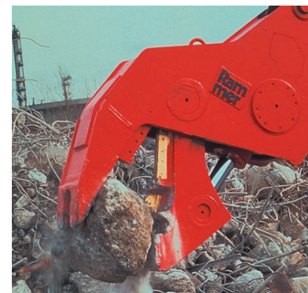
FIGURE 5.3.-5. German contractor Bavak, Bauschutt and Holzverwertungsanlage Karlsruhe GmbH turns demolition waste, soil and road surfacing into grebe and chipping for reuse. Such recycled material is being increasingly used in road building and other construction purposes. Bavak has used its Rammer RB 28 pulverizer since 1994. It is used to remove steel reinforcement from concrete debris brought to the site. The treated concrete is then fed into a crusher for recycling.
