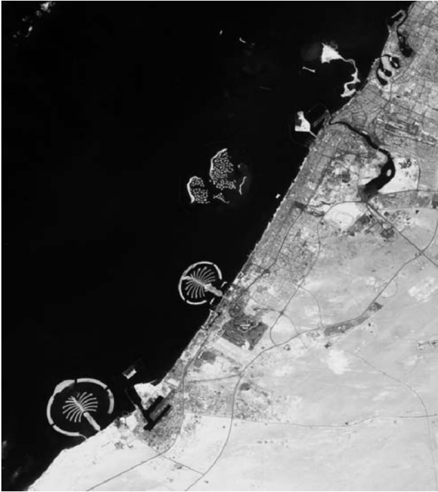
Figure 1.1 Man-made archipelago in Dubai, United Arab Emirates. Groups of islands in the shape of palm trees have been constructed by building up the seabed with material dredged from elsewhere. The palm islands are called Palm Jebel Ali, Palm Jumeirah and Palm Deira, respectively, from the south to the north. The largest island, Palm Deira, was just being started (towards the top right) when this image was taken. Between Palm Jumeirah and Palm Deira there is ‘The World’, a cluster of 250–300 small islands in the shape of a world map. The ASTER image was acquired on 18 September 2006, is centred near 25.3°N, 55.3°E, and covers an area of 46.1 × 57 km. This image is reproduced with acknowledgement to the NASA/GSFC/METI/ERSDAC/JAROS, and US/Japan ASTER Science Team.
