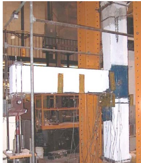
b) Specimen TR2 (8 GFRP sheets on the underside of the beam and column with corner steel angle 500x225x225x8 mm connected to beam with 8 steel bolts 20 mm dia and sandwiching column with 500x200x25 mm back steel plate using 4 steel rods 25 mm dia. 3 mm thick U-shaped steel plates are used in beam and 2 steel plates 320x100x12 mm with 4 steel rods 12 mm dia. are used in column )
