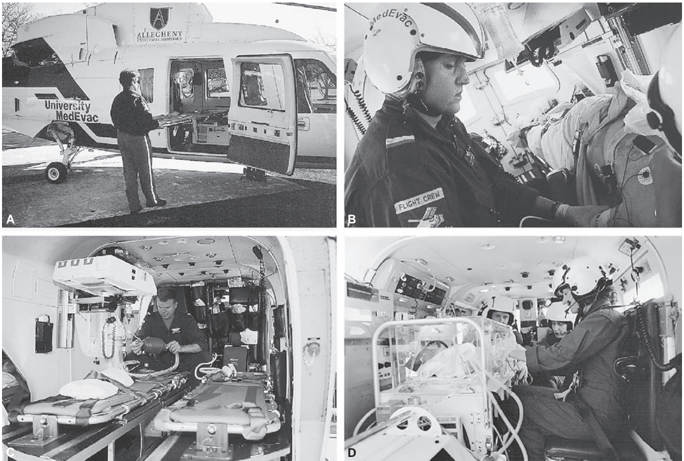
FIGURE 6.5 A–D: Air medical transport environment. Examples of design of a medical helicopter (“rotor-wing”). Note relative space and patient access limitations. (A–C: From Hahnemann University Hospital, University MedEvac, Philadelphia, PA, with permission; D: Used with permission, © The Children’s Hospital of Philadelphia, Philadelphia, PA.)
