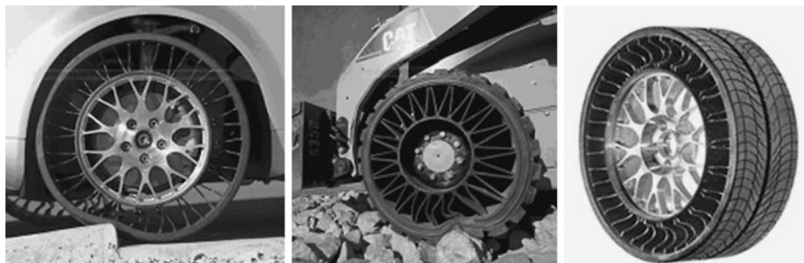
Fig. 4.10 The ‘twheel’ by Michelin, an airless tire being developed for automotive applications
