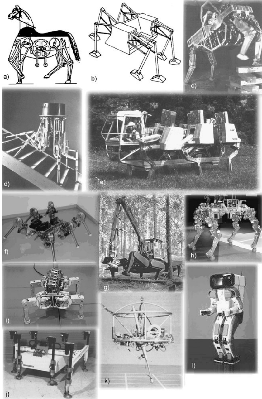
Fig. 6.1 A selection of images of walking devices; (a) Walking Horse; (b) Iron Mule Train; (c) General Electric Walking Truck; (d) Odeics Functionoid; (e) Ohio State University Adaptive Suspension Vehicle; (f) University of Karlsruhe Lauron II; (g) Plustech; (h) University of Karlsruhe Bisam; (i) Tokyo Institute of Technology Titan VIII; (j) Martin Marietta Walking Beam; (k) Carnegie Mellon Hopper; (l) Honda humanoid robot
