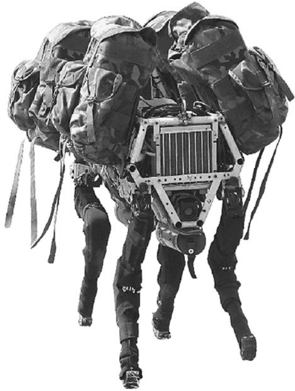
Fig. 6.15 The Big Dog, one of the few successful walking machine able to achieve a true dynamic stability
