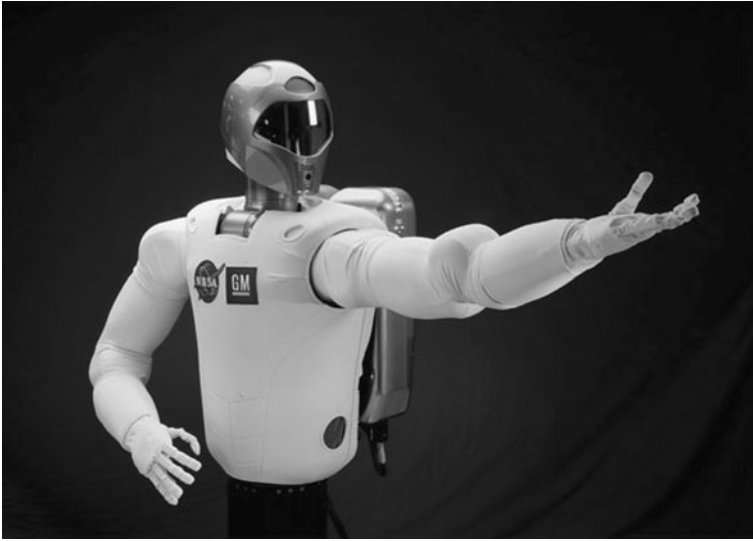
Fig. 3.5 The NASA Robonaut has two anthropomorphic arms provided with human-like hands (NASA image)
