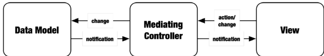
Figure 20-3. Mediated Model-View-Controller design pattern
