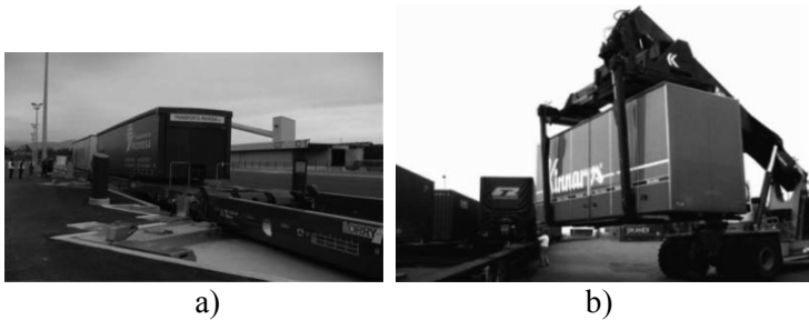
Figure 4.21. Combined transport systems. a) A piggyback train [MOD]; b) a transshipment swap body http://www.modalhor.com/
