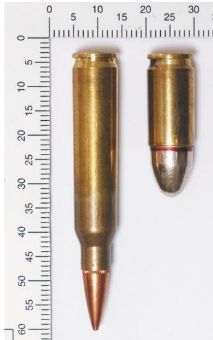
Figure 23.18 A 9 × 19 mm Luger semi-automatic pistol cartridge (top), and a NATO 5.56 × 45 mm automatic rifle cartridge (bottom).
