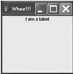
Figure 16-14. Our label is now centered in the NORTH region of the JFrame.
