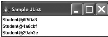
Figure 16-21. Relying on the default toString method yields a less cosmetically desirable result.
