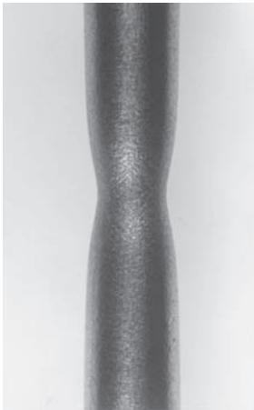
FIGURE 6.7 Neck down of a tensile test specimen within its gage length after extension beyond the tensile strength. (Courtesy of R. S. Wortman.)
