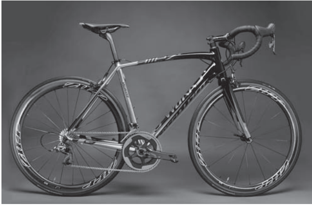
This elegant road bike uses a carbon-fiber reinforced polymer composite to provide optimal performance. (© Hugh Threlfall / Alamy.)
