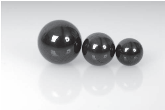
Modern ceramics can display excellent wear resistance. This property is used to full advantage in these \text{Si}_3\text{N}_4 bearing balls. (© David Page photography / Alamy.)
