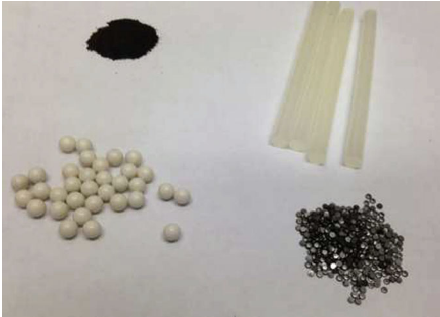
Fig. 1.1 Typical printing ingredients: top left: finely ground metallic powder (iron). Top right: extruded PLA. Bottom left: ABS pellets and bottom right: coarsely ground steel flakes
