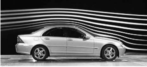
FIGURE 10.1 Smoke-traced streaklines of flow around a car. (Source: DaimlerChrysler.)
