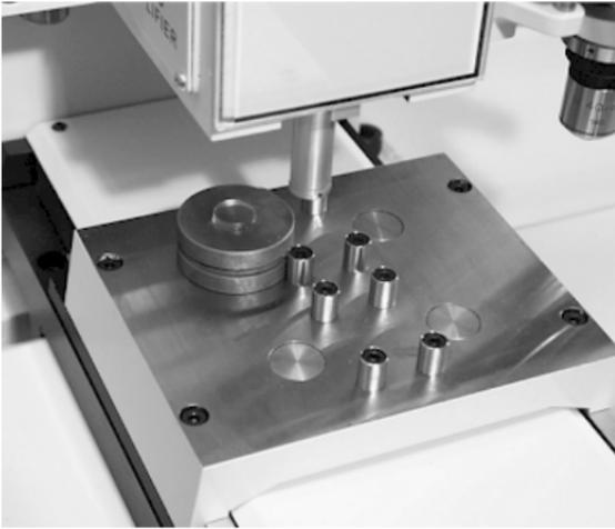
**Fig. 2.8** Example of a fused silica specimen mounted on a cylindrical hardened steel magnetic specimen mount and placed into position on a servo-motor-driven X-Y positioning stage. In this instrument, there is provision for four specimen mounts on the stage with powerful magnets mounted beneath each position to firmly clamp the specimen holder to the stage (Courtesy CSIRO).
