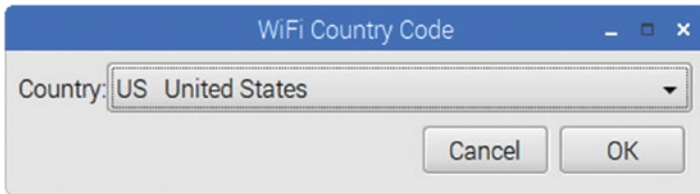
Figure 4-18. Use the WiFi Country Code dialog box to set the Wi-Fi standard that the Raspberry Pi is using.
