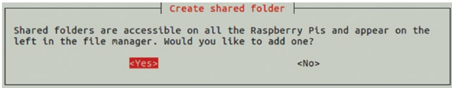
Figure 7-38. In the Create Shared Folder dialog box, select the Yes button and press the Enter key.
