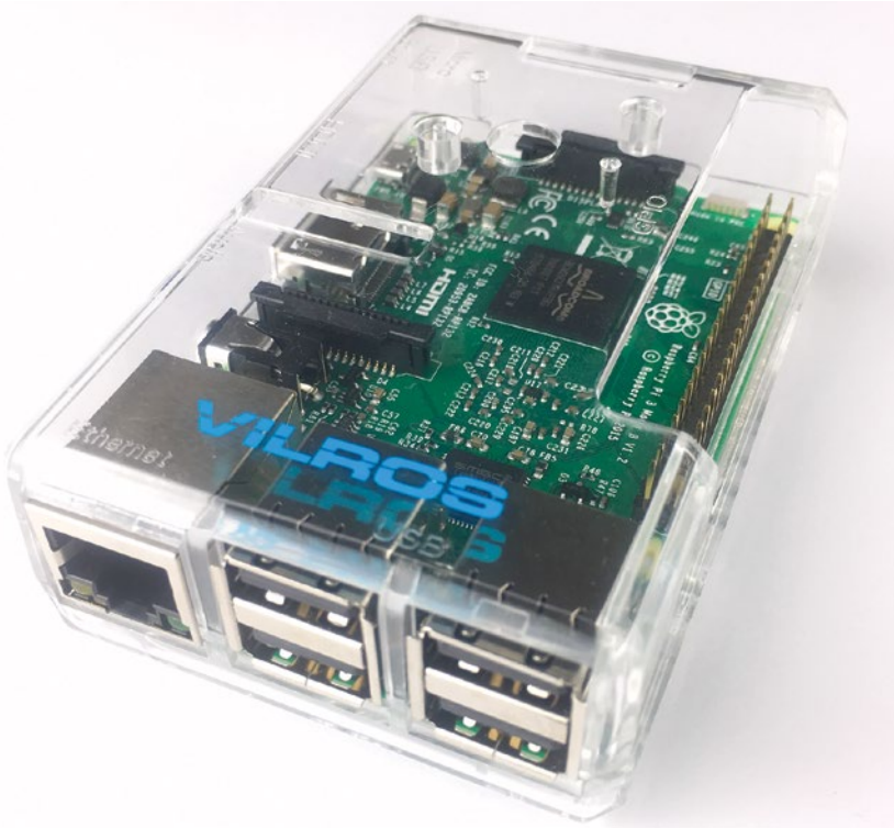
Figure 1-2. You can get a wide variety of cases for the Raspberry Pi models including clear cases and ones that give easy access to the internal ports.
