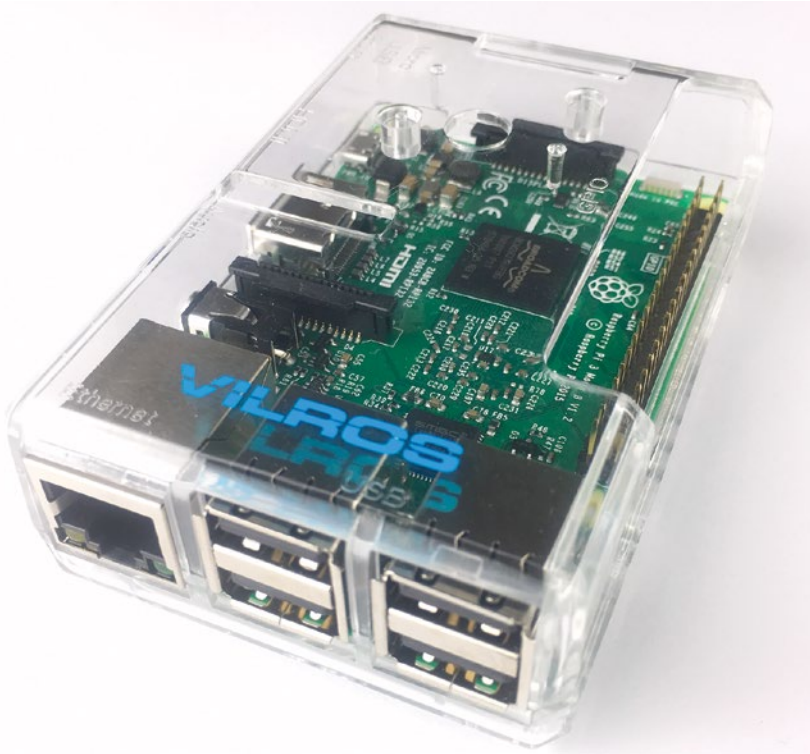
Figure 2-10. Acrylic cases enable you to admire the Raspberry Pi’s components as you compute. This Vilros Clear Case has a cutout that gives access to the GPIO pins.
