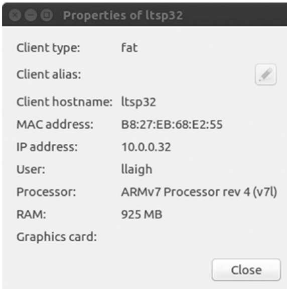
Figure 7-59. The Properties dialog box lets you see a client's type, MAC address, processor type, and other details.
