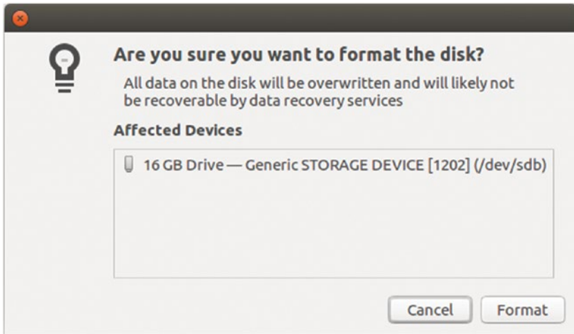
Figure 5-9. In the confirmation dialog box, verify that you've selected the right disk, and then click the Format button.
