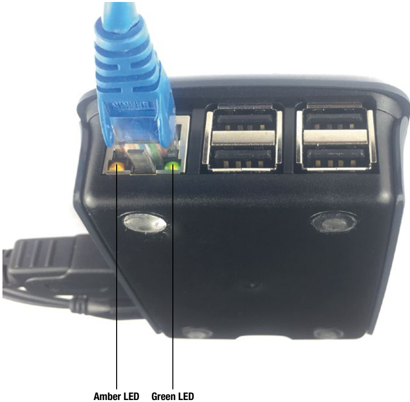
Figure 8-4. You can use the amber LED and the green LED in the Ethernet port to determine whether a Raspberry Pi computer has a working network connection.
