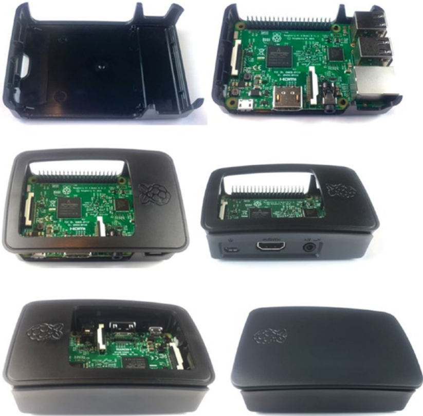
Figure 5-1. The official Raspberry Pi case for the Raspberry Pi 3 Model B clips together in six easy steps.
