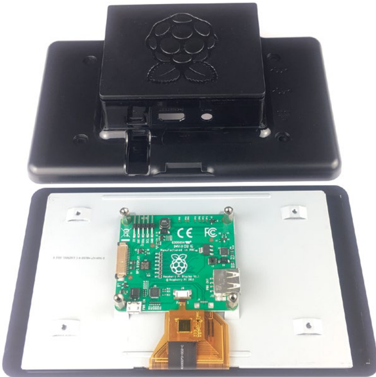
Figure 2-11. Touch screen cases, such as the Premium Case for Raspberry Pi 7" Touch Screen (top) enable you to turn a touch screen, such as the Raspberry Pi 7-Inch Touch Screen Display (bottom), into a tablet computer.
