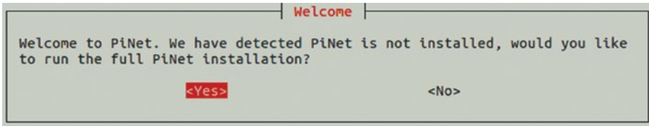
Figure 7-16. Select the Yes button and press the Enter key in the Welcome dialog box to start installing PiNet.
