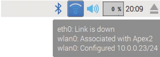
Figure 6-7. Once the Wi-Fi connection is established, the Wi-Fi Networks icon appears as a Wi-Fi symbol. You can hold the pointer over the icon to display a pop-up balloon showing the Wi-Fi network and the IP address.
