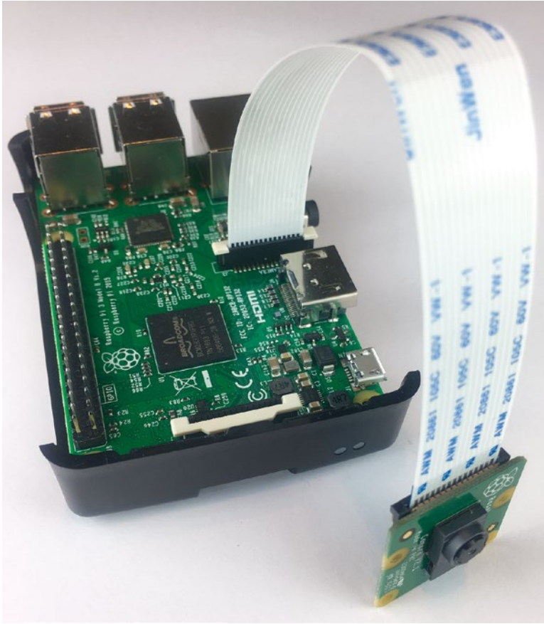
Figure 2-12. Connect a camera module to a Raspberry Pi computer when you need to get graphical input.
