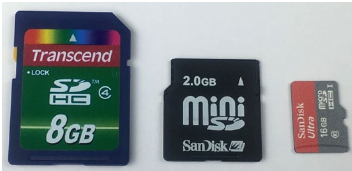
Figure 2-6. A standard SD card (left), a mini SD card (middle), and a micro SD card (right)
