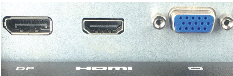
Figure 2-13. DisplayPort (left), HDMI (center), and VGA (right) ports on a monitor
