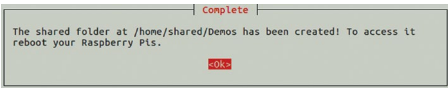
Figure 7-41. The Complete dialog box confirms that you have created the folder and reminds you to reboot the Raspberry Pi computers to access it.
