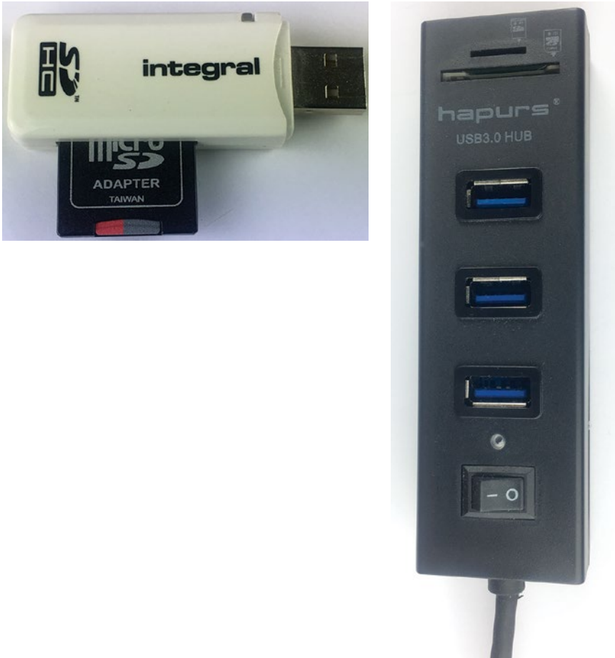
Figure 2-7. A USB stick-type SD card reader (left) is handy and portable, but a desktop card reader (right) is easier to use for heavy-duty work with SD cards.
