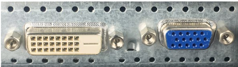
Figure 2-14. DVI (left) and VGA (right) ports on a monitor
