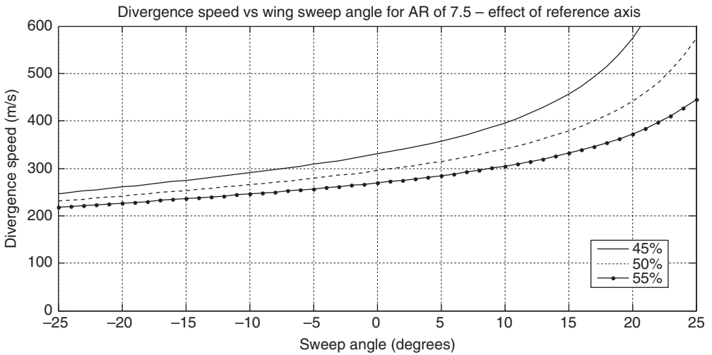
Figure 7.11 Effect of sweep angle on divergence speed for different reference axis positions.
