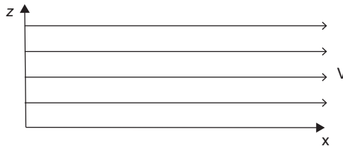
Figure 18.1 Uniform flow streamlines.
