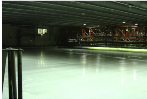
Figure 12.5 Model testing of ice–structure interaction.
