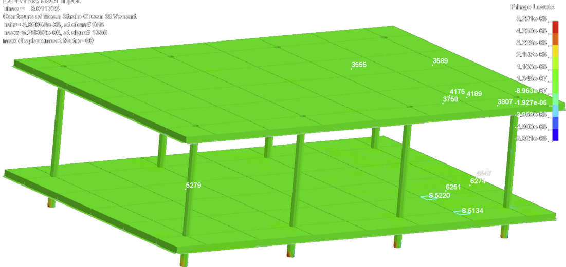
Figure 49.20 The strain distribution at 0.12 s.
