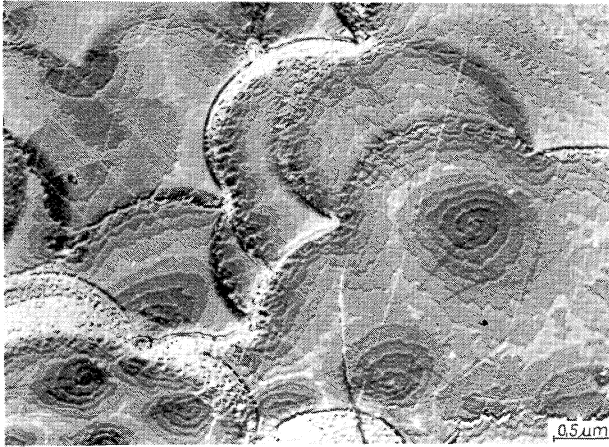
Fig. 5 : Transmission electron micrograph of an Au(111) film epitaxially grown on a (111) Ag substrate.
