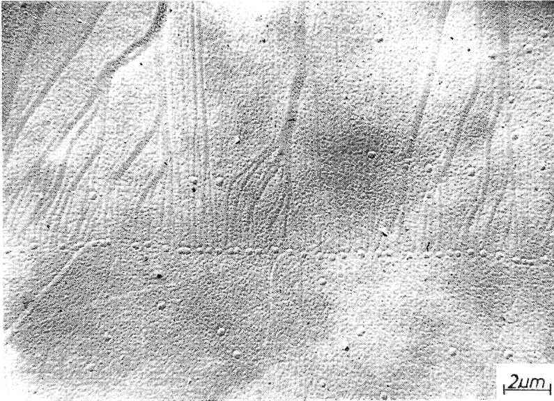
Fig. 2 : Development of monatomic steps on an NaCl (100) cleavage face due to NaCl evaporation.
