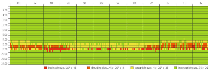
Fig. 2 Example of the output of a simulation for glare on a room over one year
