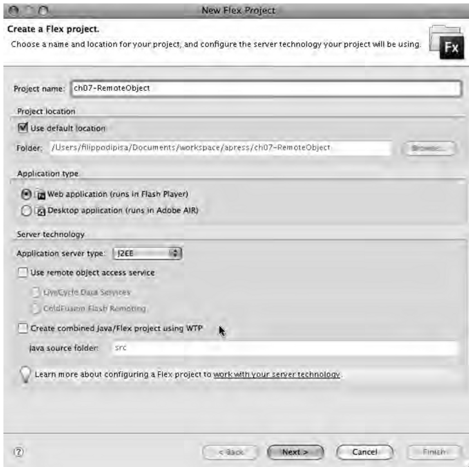
Figure 9-20. New Flex Project dialog box with the server technology set to use Java EE as remote server
