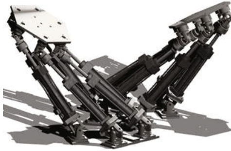
Figure 7: 3D projection of the mechanical design of the normal gait simulator based on the Stewart-Gough platform
