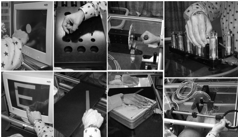
Fig. 3 - The AutoCITE consists of eight instrumented task devices. Reproduced from Taub et al. (2005) (65) with permission.
