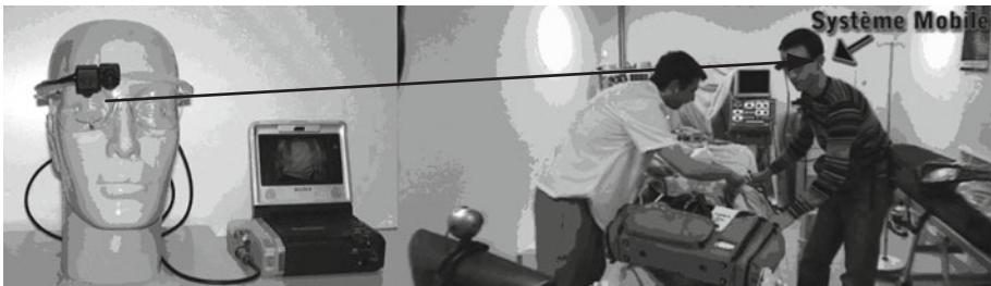
Fig. 7 - A mobile eye tracker used with the full-scale simulator SimMan.
