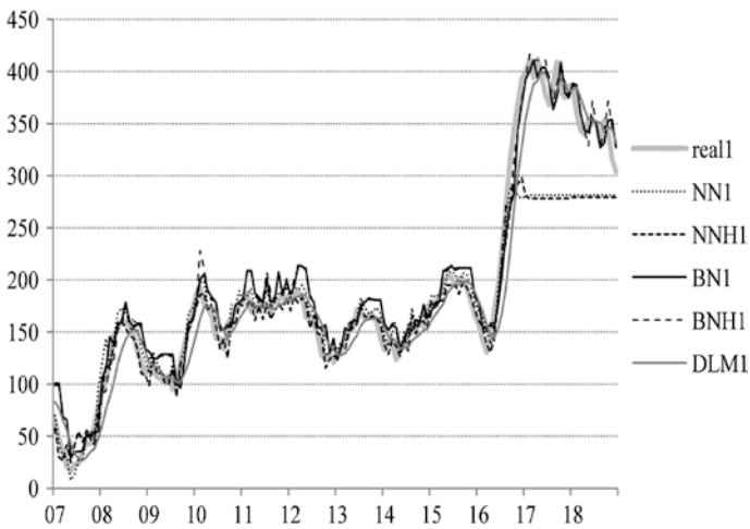
Fig. 15 One step forecast 27.11.2011 (Sunday), the scale is changed due to lower traffic volume
