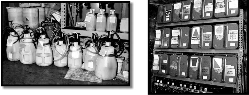
FIGURE 7.13 Example of color and shape coded transfer equipment.
