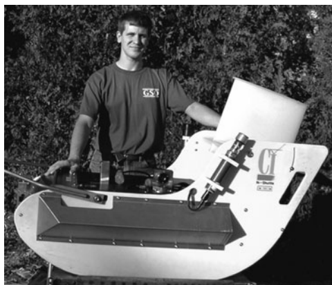
Fig. 4.5. NuShuttle, an undulating oceanographic sampling platform, carries sensors for temperature, salinity, chlorophyll, primary productivity and dissolved oxygen. The shuttle also contains a Continuous Plankton Recorder (CPR) mechanism.
