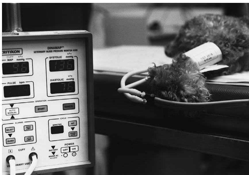
FIG. 2.13 The DINAMAP 8300 (Sharn, Tampa, Florida, USA) utilizes the oscillometric method of measuring arterial blood pressure non-invasively.
