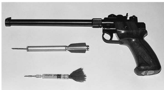
FIG. 17.3 'Dist-Inject' dart pistol with projectile syringe. The lower illustration is of the 'Miniject' projectile syringe for use with a blowpipe.
