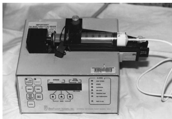
FIG. 15.8 Syringe driver (Medex Inc., Duluth, Georgia, USA) for continuous administration of propofol or other anaesthetic agents or fluids.
