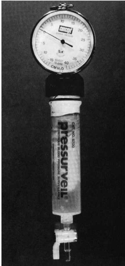
FIG. 2.18 Pressure transfer unit in which a latex diaphragm isolates the aneroid manometer from the fluid-filled catheter line. These units are presterilized and disposable.
