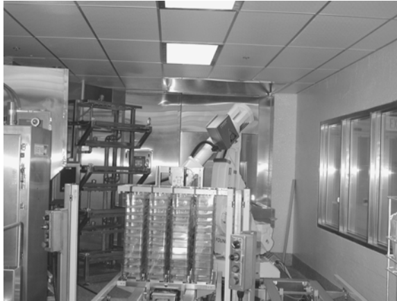
Figure 8.24 A robot stacking clean bedded cages four at a time after having picked the cages off of the indexing tunnel washer belt in back of the robot and placing them under a bedding dispenser that is pneumatically fed from a larger bedding storage hopper located near the dock where bedding is received. The cages are being stacked on special carts that rest on rails, all designed to precisely align the stacks of cages. On the soiled side, an identical combination of robot, carts, and rails are used to load soiled cages onto the tunnel washer belt after the robot dumps the soiled bedding into a hopper, from where it is pneumatically transported to a disposal container outside the facility.
