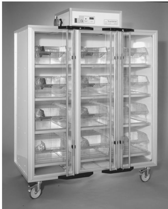
Figure 11.9 A ventilated cabinet for maintenance of laboratory animals (Scanbur, Denmark).
