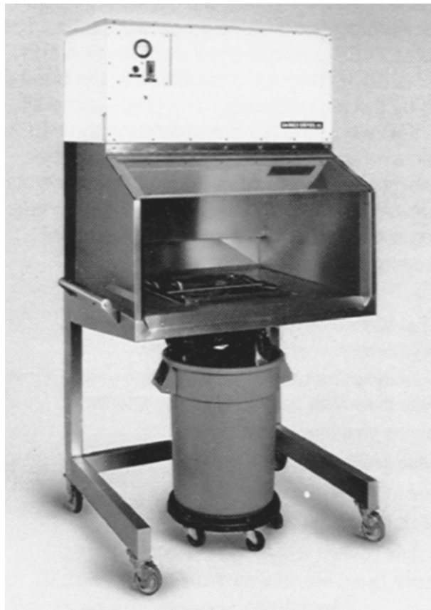
Figure 8.4 Shown is a soiled bedding dumping station that uses mass air displacement to contain bedding dust, drawing it away from the operator standing in front of the cabinet, while dumping soiled bedding from a cage inside the cabinet. The air draws the dust into the back of the cabinet, where it is filtered out from the air that is first passed through a coarse filter and then a HEPA filter before being returned to the room. (Courtesy of Allentown Caging Systems Co., Inc.)
