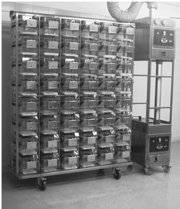
Figure 8.19 An individually ventilated microisolation cage rack with two filter and blower units mounted on a mobile rack alongside the cage rack. The cage exhaust filter and fan unit is connected directly to the room exhaust at the ceiling, similar to that shown in Figure 8.16 .
