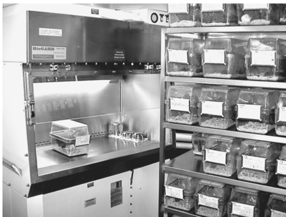
Figure 8.27 A rack with static microisolation cages adjacent to a Type II A biosafety cabinet with a microisolation cage inside the cabinet. The combination of the microisolation cage and cabinet makes up what is known as a “microisolation cage system.” The microisolation cages are only opened inside the cabinet, including for cage changes or research procedures.
