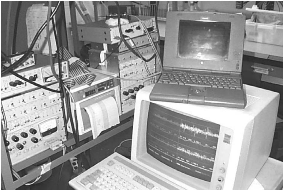
Figure 56.2 Example of a data acquisition system. The biological signals from the fetus are recorded digitally to the computer aided system for further analysis.
