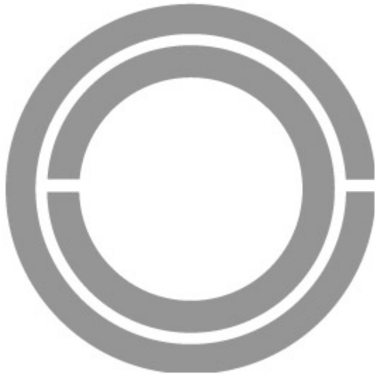
Figure A2.2: A doubly split metallic ring as a metamaterial element. Dimension in the third dimension is usually small. The metal is evaporated in a substrate.
