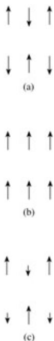
Figure 11.19: The angular momentum vector for (a) antiferromagnetic, (b) ferromagnetic and (c) ferrimagnetic materials.
