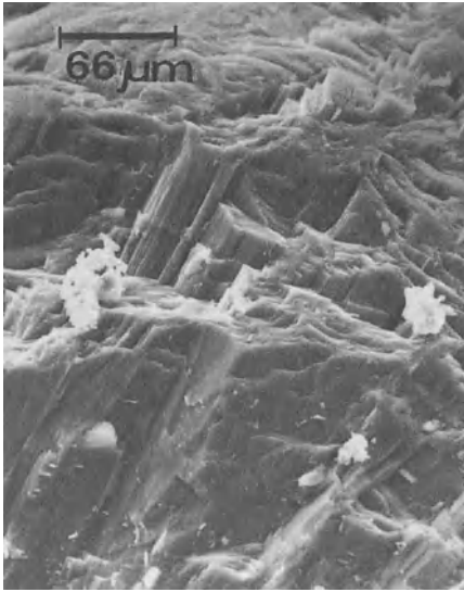
Fig. 40. Whewellite showing columnar texture (SEM)
