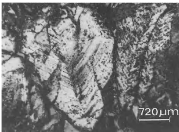
Fig. 55. The growth bands of struvite grains, see Fig. 45 (polarizers uncrossed).
