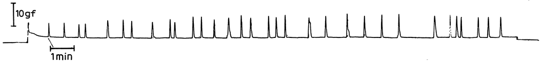
Fig. 5. Measured stress relaxation curve with superimposed spontaneous contractions. Time runs from left to right
