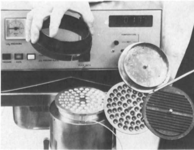
Fig. 6. Interchangeable plates for freezing in pellet form or straws and in alcohol bath (model CSF 16)
