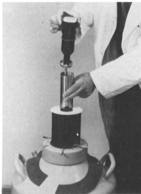
Fig. 2. Sherman's modification BF 5 biological freezer (accessory part to the duer LR 30): a the neck tube plug; b freezer core assembly; c receptacle for straws and ampoules are placed in the container over the liquid nitrogen level
