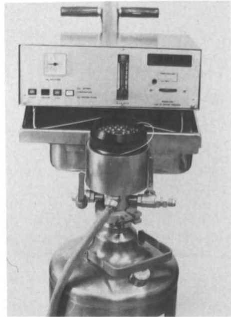
Fig. 4. The semiautomatic sperm freezing device (model CSF 16 Ricor DTD, Kibutz Ein Harod, Barkay and Zuckerman 1978 c)
