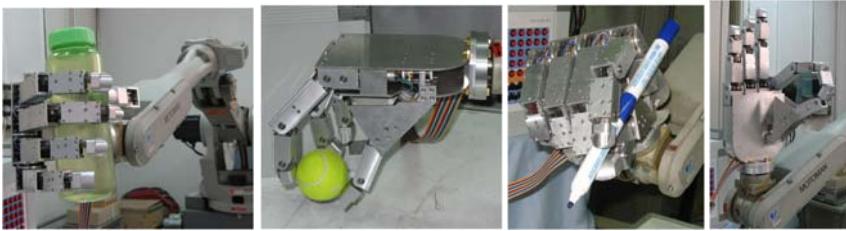
Fig. 9. GCUA Hand grasping different objects
