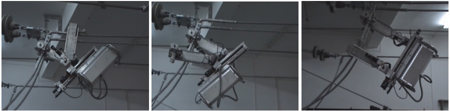
b) The robot moves from the horizontal line to the jumper
