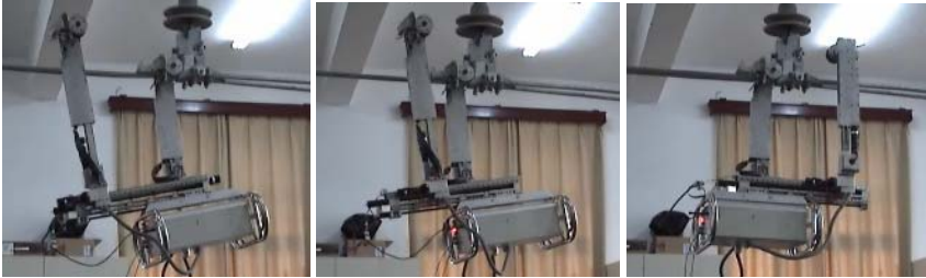
a) The robot crosses the insulation string on horizontal line
