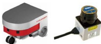
Fig. 1. Left: robuLAB80 mobile robot used in the experiments Right: Hokuyo laser
