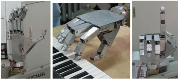
Fig. 10. Operations and poses of the GCUA Hand
