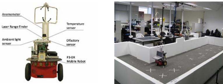
Fig. 5. The mobile robot with its sensors (left) and the environmental setup (right). The dimensions of the L-shaped environment are given in Fig. 6 (in mm).
