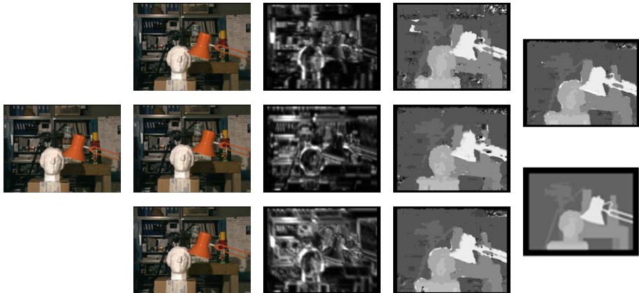
Fig. 3. Algorithm's Steps and Results for the Tsukuba Data Set. (Column 1) the Reference Image (Up-Left), (Column 2) the Three Target Images (Up-Right, Down-Left, Down-Right), (Column 3) the Certainty Maps for the Horizontal, Vertical and Diagonal Pair, (Column 4) the Computed Disparity Map for Each Stereo Pair, (Column 5) the Fused (Top) and the Ground Truth (Bottom) Disparity Maps.
