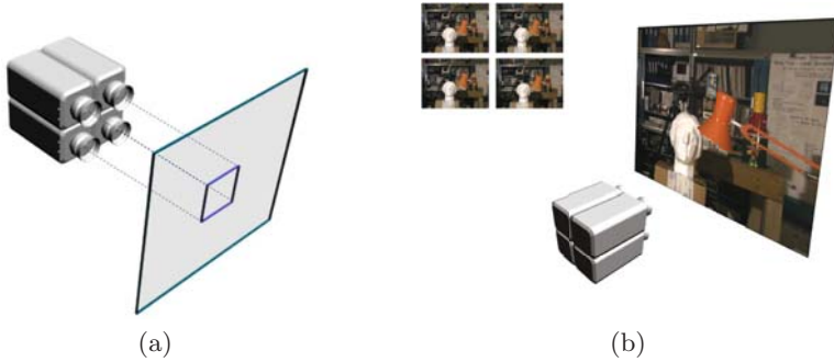
Fig. 1. (a) The Quad-camera Configuration and (b) the Results (Up-Left) and Scene Capturing (Right) Using a Quad-camera Configuration
