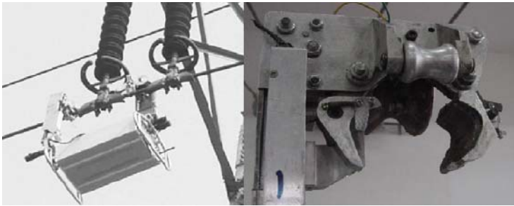
Fig. 1. The power line robot and the structure of its arm
