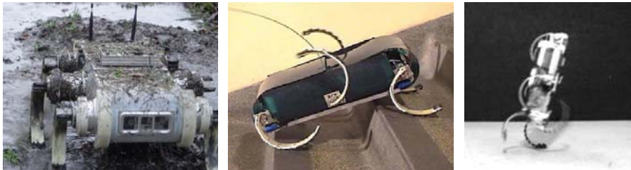
Fig. 1. RHex's versatile locomotion. Left: Walking on mud. Middle: Climbing stairs. Right: Bipedal walk.
