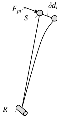
Fig. 2. The flexibility deformation of RPS leg
