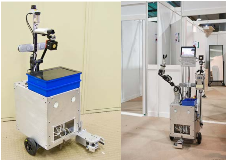
Fig. 1. RH4-Y, version 4 of our cooperating robot for applications at home (photos HEIG-VD / PFG)
