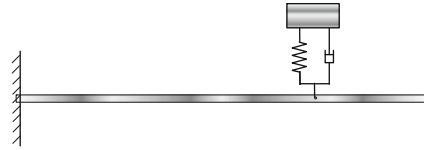
Fig. 5.52 A cantilever beam with an appended system
