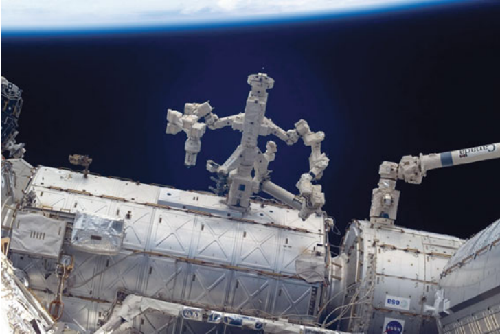
Fig. 10.1 The special purpose dexterous manipulator (SPDM), also known as dextre telemanipulator, at work on the international space station (ISS). Canadarm or RMS is also seen in the picture (Source NASA, http://www.nasa.gov/images/content/287299main_dextre_iss017_big_full.jpg )
