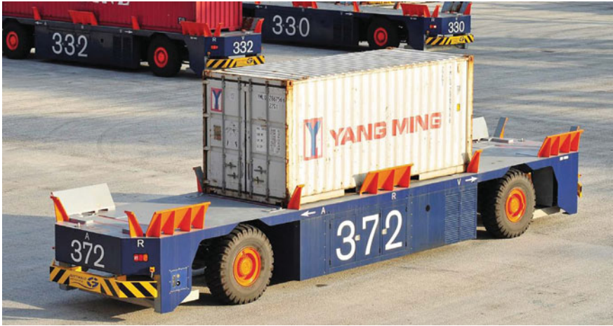
Fig. 11.3 Horizontal container transport using AGVs in the ECT Euromax terminal, port of Rotterdam (Netherlands). Courtesy of: Gottwald Port Technology GmbH [7]
