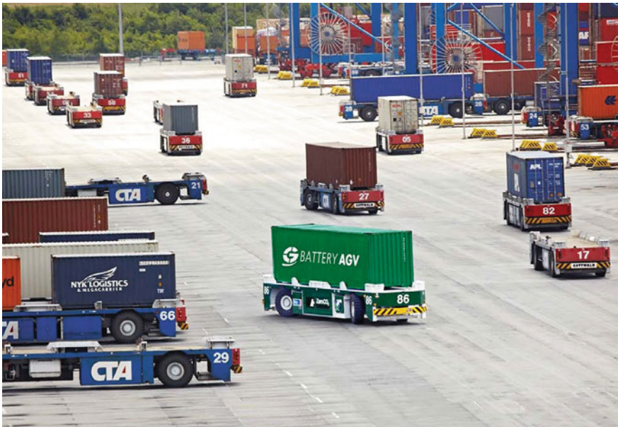
Fig. 11.4 Battery-driven AGV in the CTA terminal, port of Hamburg (Germany), operating in a fleet of diesel-electric AGVs. Courtesy of: Gottwald Port Technology GmbH [7]
