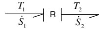
Fig. 3.77 Heat transfer at constant gas mass modeled as an R-field with two-ports
