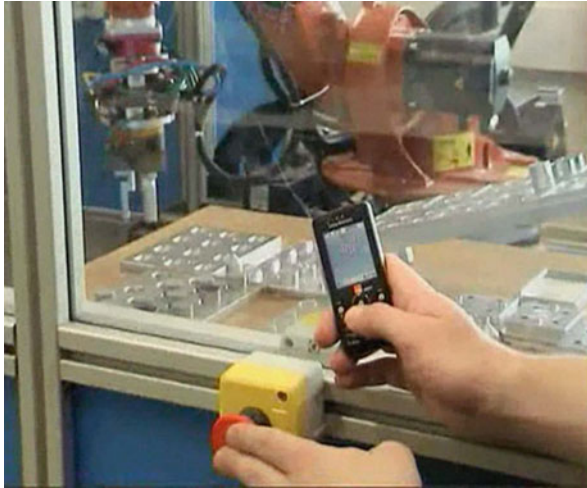
Fig. 12.2 Teledetection of robot input–output using mobile phone
