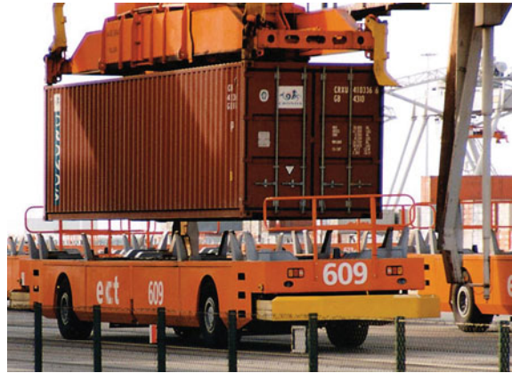
Fig. 11.2 Gottwald AGV in the ECT Delta terminal, port of Rotterdam (Netherlands), during loading. Courtesy of: Gottwald Port Technology GmbH [7]
