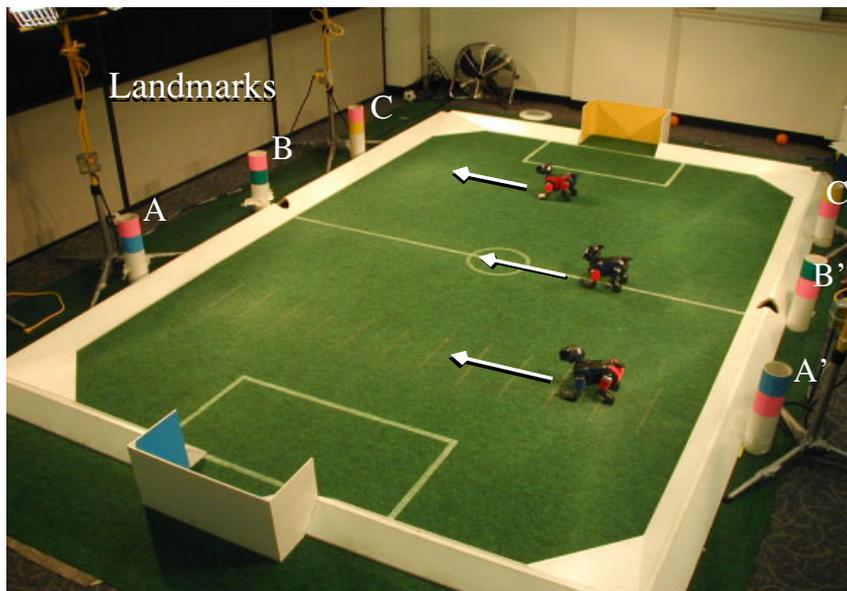
**FIGURE 5.6:** The training environment for the gait learning experiments. Each AIBO times itself as it moves back and forth between a pair of landmarks (A and A', B and B', or C and C').
