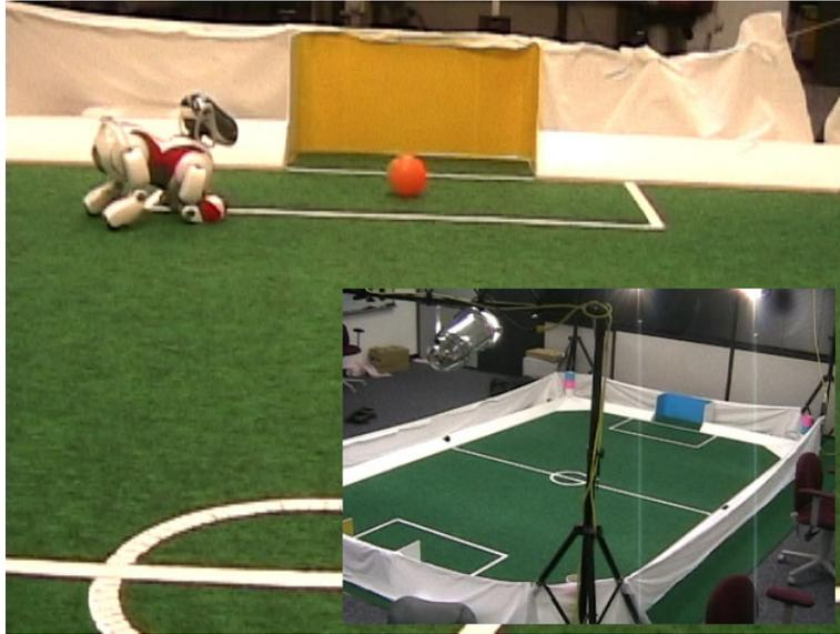
**FIGURE 1.1:** An image of the AIBO and the field. The robot has a field-of-view of  $56.9^\circ$  (hor) and  $45.2^\circ$  (ver), by which it can use the two goals and four visually distinct beacons at the field corners for the purposes of localization.
