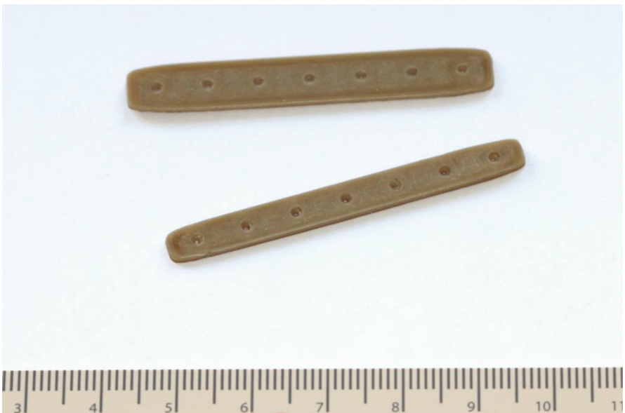
Fig. 1. 3D-printed PEEK osteosynthesis plates (length of 50 mm)
