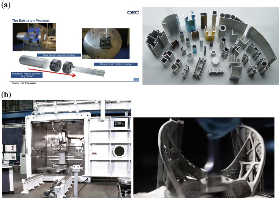
Fig. 1. (a) Extrusion process (left) and products (right) (b) Biggest 3D printer (left) and manageable complexity of product design (right)
