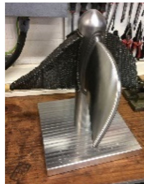
Fig. 15. CNC machined blade of Design #2
