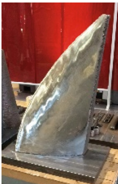
Fig. 14. Ground face of Design #1 and #3.
