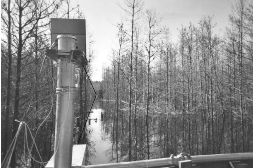
Fig. 3.10. FLUDEX-ELA experimental reservoir No 1, dual-beam infrared laser monitoring site of CO 2 and CH 4 , optical path of 340 m (forward and backward), August 2001
