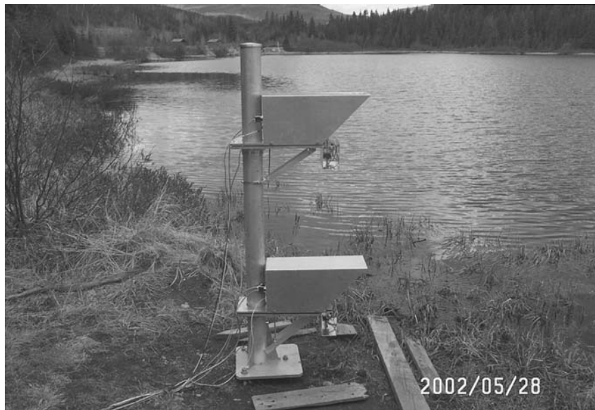
Fig. 3.2. Experimental set-up of the laser tower for dual beam measurements
