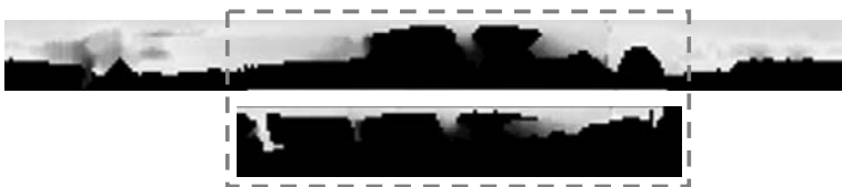
Fig. 5 DGI-BS representation of a non-occluded object (above) and DGI-BS representation of the same object under occlusion circumstances placed in the best matching position (below).
