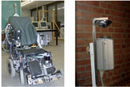
Fig. 1 Left: the wheel chair test platform. Right: the omnidirectional camera system.
