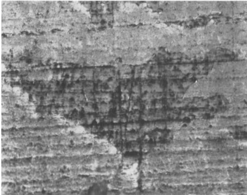
Figure 12. Spalled spot of SiC coating from PG substrate.
