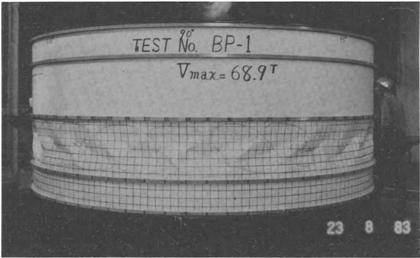
Fig.10 Buckled Shell between Ring-Stiffeners
