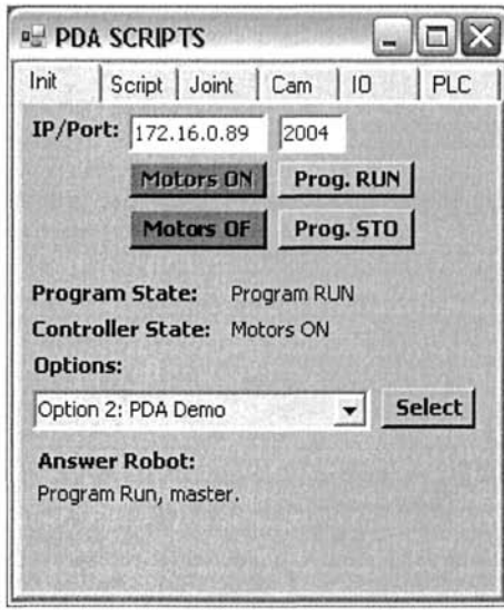
Figure 3.24 PPC screen to initialize robot operation and select program option
